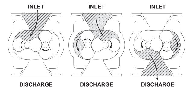
Figure 4-1 – General Operation Principle
