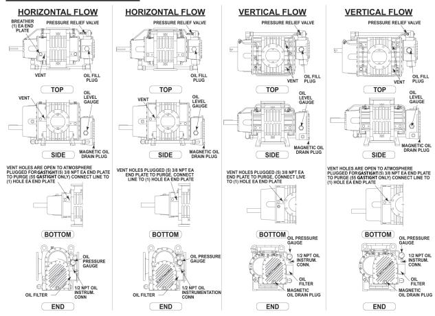
Figure 5-4 - Locations of Oil Fill, Drain, Level Gauges, and Cooling Connections on Blowers with Integral Lubrication
