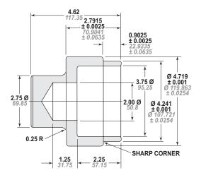
Figure 12-3 – Mechanical and Lip Seal Tool
