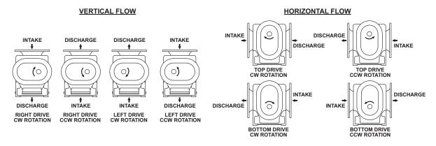
Figure 4-2 – Flow Direction by Rotation
