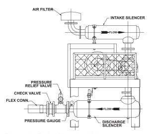
Figure 5-1 – Typical Blower Installation
