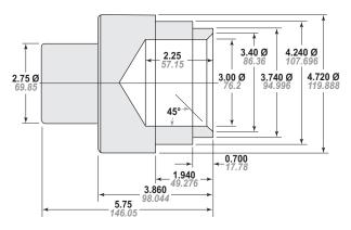
Figure 12-1 - Lab Seal Pressing Tool
