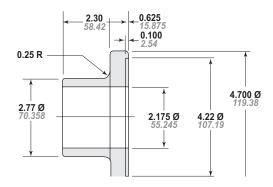
Figure 12-4 – Bearing Pressing Tool
