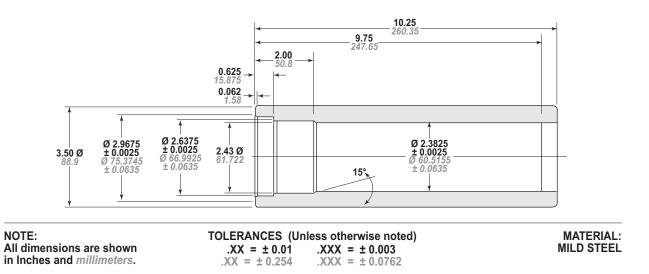
Figure 12-5 – Drive Shaft Bearing Inner Race Pressing Tool
