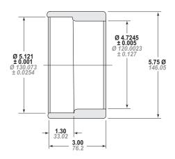
Figure 12-2 - Seal Installation Tool
