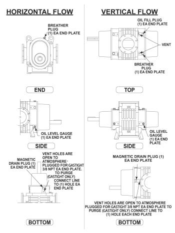
Figure 5-3 – Locations of Oil Fill, Drain, and Level Gauge on Blowers with Splash Lubrication
