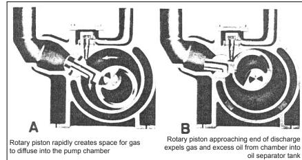
Figure 1. Operating Cycle of KDH Series Single Stage Pumps
