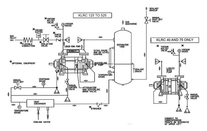
Figure 3-4 – Piping Schematic: Full Sealant Recovery System without Circulating Pump
