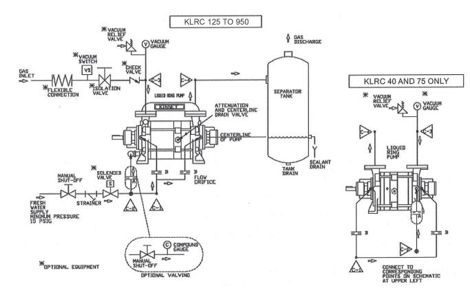
Figure 3-1 – Piping Schematic Once-Through Recovery System
