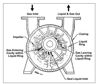
Figure 1-1 – Cross-Section Liquid Ring Pump
