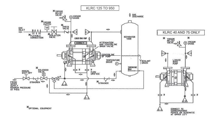
Figure 3-2 – Piping Schematic: Partial Sealant Recovery System
