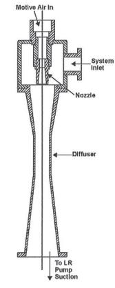
Figure 3-5 – Air Ejector
