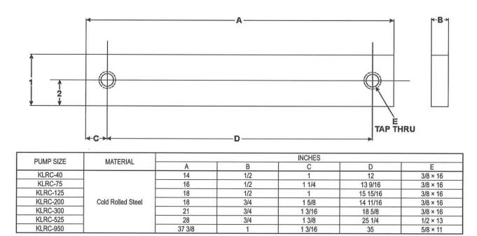
Figure 8-3 – Foot Alignment Tool
