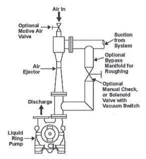
Figure 3-6 – Air Ejector Installation
