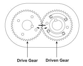
Figure 8-3 – Timing Marks Advanced 3 Teeth (Reference Marks Aligned)
