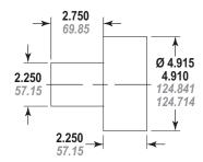
Figure 13-1 – Labyrinth Seal Installation Tool
