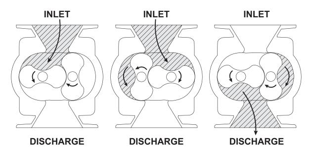
Figure 4-1 – General Operation Principle
