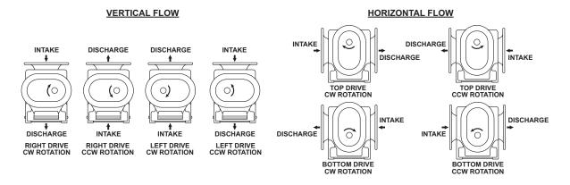
Figure 4-2 – Flow Direction by Rotation
