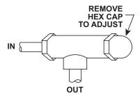
Figure 5-4 - Pressure Relief Valve
