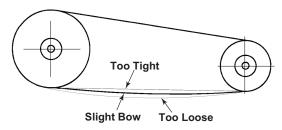
Figure 5-5 – General appearance of a V-belt drive
