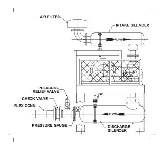
Figure 5-1 – Typical Blower Installation
