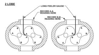
Figure 8-4 – Checking Rotor Interlobe Clearance
