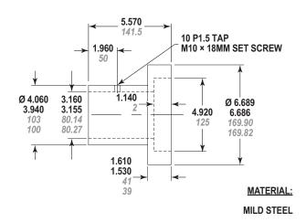
Figure 13-4 – Alignment Tool for Drive Shaft Bearing
