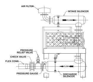
Figure 5-1 – Typical Blower Installation
