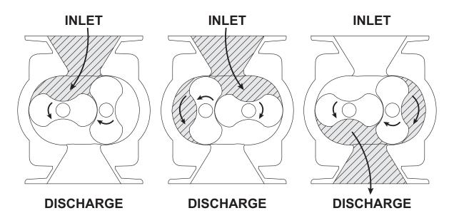
Figure 4-1 – General Operation Principle
