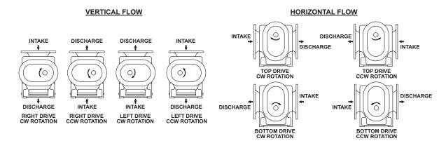
Figure 4-2 – Flow Direction by Rotation
