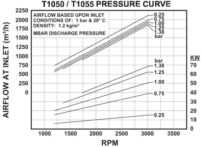
Figure 4-11 – T1050 / T1055 Pressure Curve (Metric)
