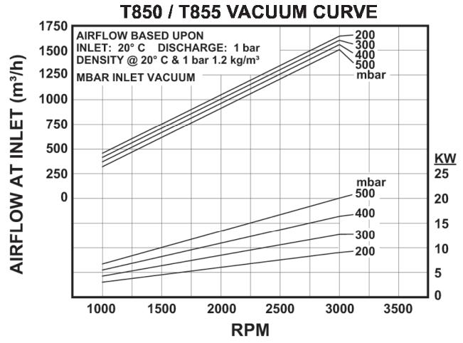
Figure 4-10 – T850 / T855 Vacuum Curve (Metric)
