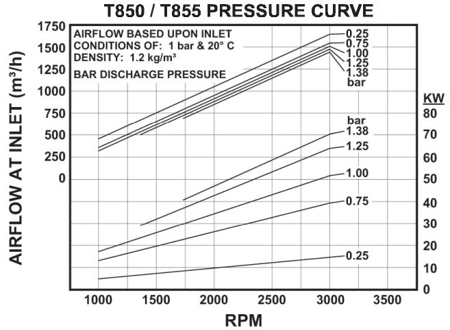
Figure 4-9 – T850 / T855 Pressure Curve (Metric)
