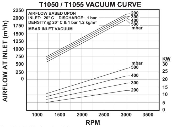
Figure 4-12 – T1050 / T1055 Vacuum Curve (Metric)
