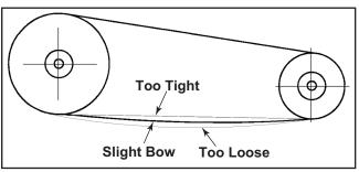
Figure 7 - General appearance of a V-Belt drive
