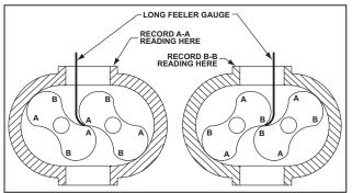
Figure 14 - Checking Rotor Interlobe Clearance
