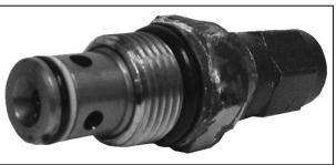
Figure 6 - Oil Pressure Adjustment Hex Cap
