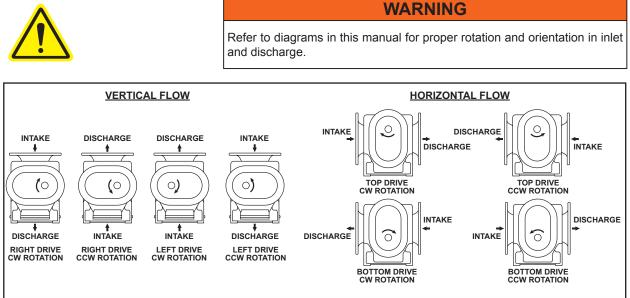
Figure 2 - Flow Direction by Rotation
