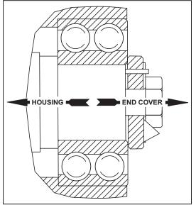
Figure 13 - Roller Bearings Illustration
