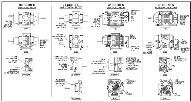
Figure 4 - Location of oil fill, drain, level gauges and cooling connections
