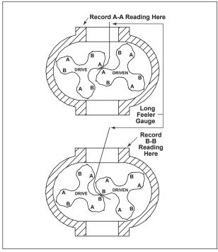
Figure 6-4 – Checking Rotor Interlobe Clearance
