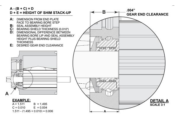
Figure 6-5 – Bearing Bore Stack-Up and Seal Measurement
