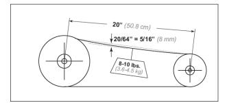
Figure 3-4 – Setting of proper tension for a V-belt drive
