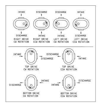
Figure 3-1 – Flow Direction by Rotation
