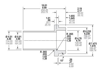
Figure 13-1 – Lip Seal Installation Tool
