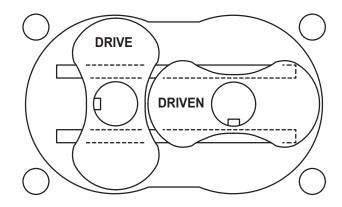
Figure 8-1 – Rotors in Housing
