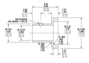
Figure 13-3 – Drive Shaft Bearing Alignment Tool
