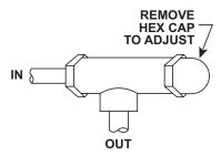
Figure 5-4 - Pressure Relief Valve
