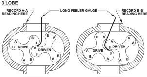
Figure 8-2 – Checking Rotor Interlobe Clearance
