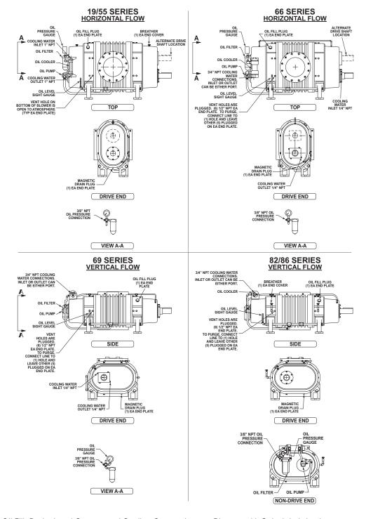
Figure 5-3 – Oil Fill, Drain, Level Gauges and Cooling Connections on Blowers with Splash Lubrication
