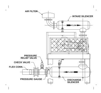
Figure 5-1 – Typical Blower Installation
