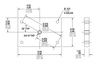
Figure 13-2 - Bearing Pressing Fixture Tool
