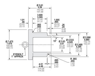
Figure 13-4 – Labyrinth Seal Installation Tool
