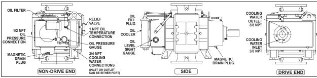
Figure 4 - Location of oil fill, drain plugs, level gauges and cooling connections
