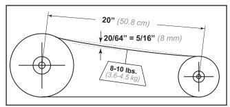
Figure 7 - Setting of proper tension for a V-Belt drive
