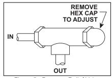
Figure 5 - Pressure Relief Valve
