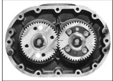
Figure 11 - Timing marks advanced 3 teeth (Reference marks aligned)
