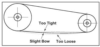
Figure 6 - General appearance of a V-Belt drive
