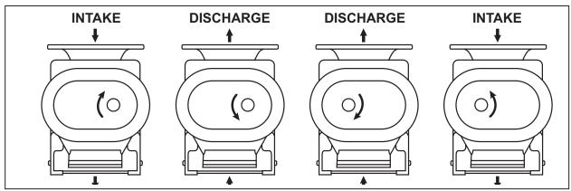
Figure 2 - Flow Direction by Rotation
