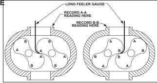
Figure 9 - Rotor Interlobe Clearance
