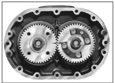
Figure 10 - Keyways in line and timing marks matched
