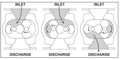
Figure 1 - Illustration of general operation principle
