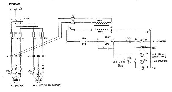
Figure 3 Typical wiring diagram, Vapor Handling System
