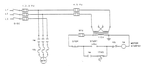
Figure 2 Typical wiring diagram Close-Coupled Booster System
