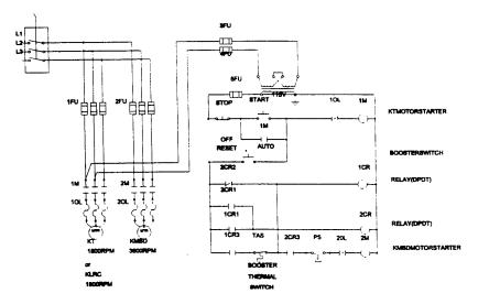
Figure 1 Typical wiring diagram, KMBD/KT, CB & KMBD/LR
