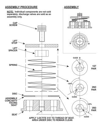
Figure 8-1 – Discharge Valve
