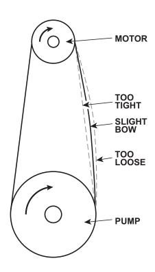
Figure 8-4 – V-Belt Tensioning
