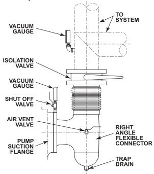
Figure 5-1 – Detailed Manifold Arrangement
