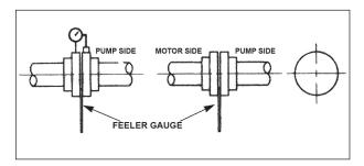
Figure 3-3 - Coupling Alignment
