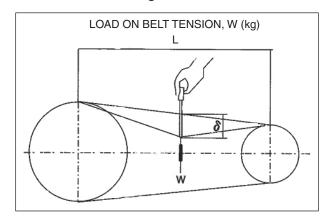
Figure 3-2 – V-Belt Tension
