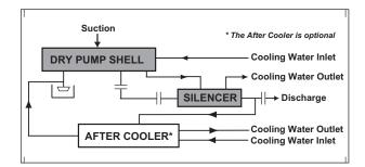
Figure 3-1 – Standard Piping
