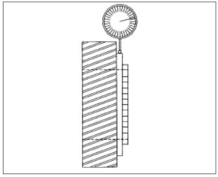
Figure 7-41 – Gear Flatness Check
