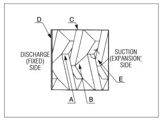
Figure 7-40 - Screw Clearance
