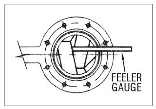
Figure 7-42 – Screw Clearance via Inlet
